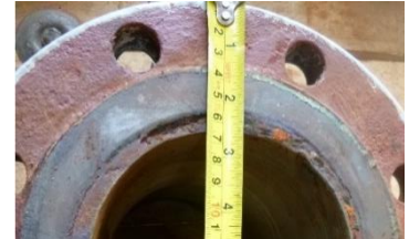
Left: scan plan of flange Inspection. Right: Crevice corrosion detected with PAUT which was later repaired
