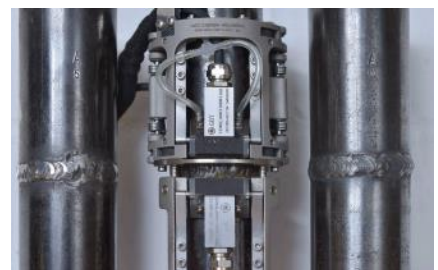
PAUT small bore pipe scanner
