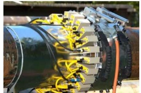
*LRUT on a high temperature pipeline*
