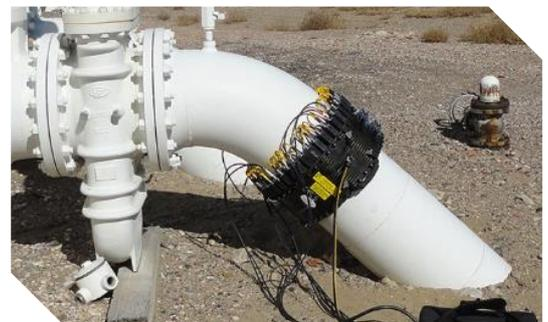
*LRUT being used to inspect a buried section of pipeline*
